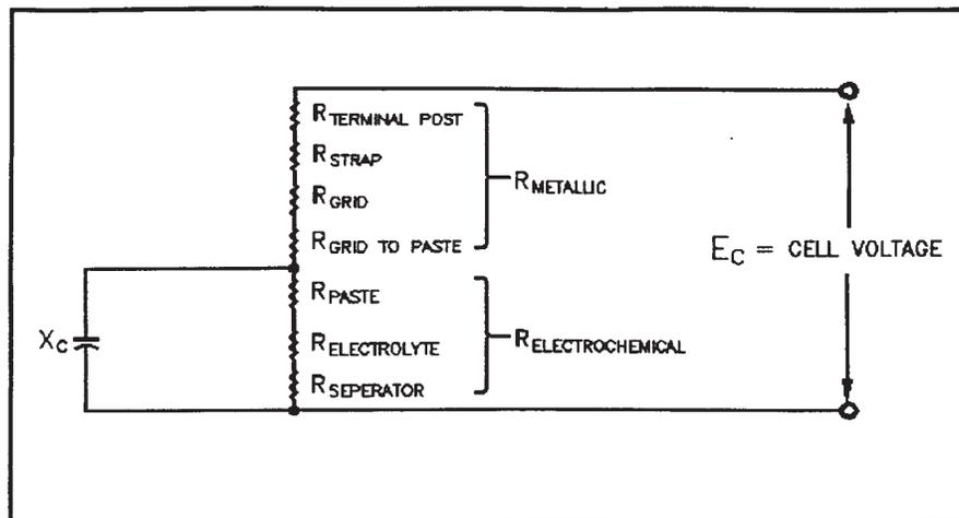
Figure 1: Simplified Model of a Lead-Acid Cell.
