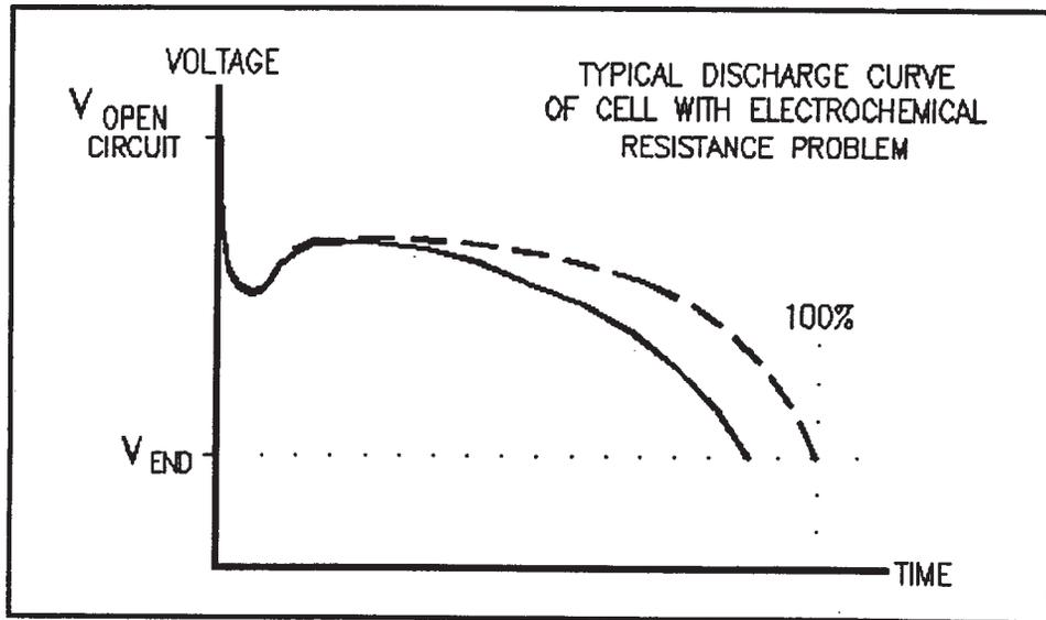
Figure 5: Typical Discharge Curve - Electrochemical Resistance Problem.
