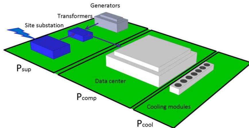
Figure 1 – Power usage in a data center
