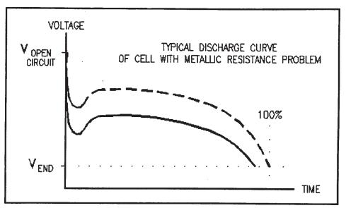
Figure 4: Typical Discharge Curve - Metallic Resistance Problem.
