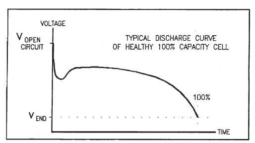
Figure 3: Typical Discharge Curve - Healthy Cell.
